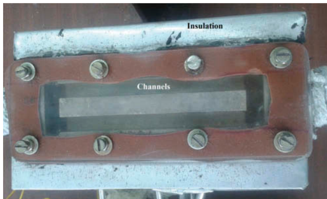
Figure 2. Aluminum block with rectangular channels.
