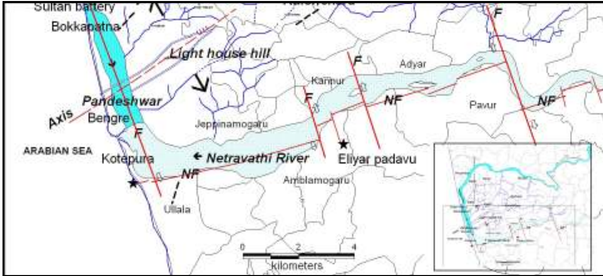
Figure 5: Present Configuration of the River Netravathi: West Flowing River Netravathi is dominantly controlled by an EW Netravathi Lineament Fault. Structural disturbances in the NNW-SSE Trending Transform (Strike Slip) Lateral Faults Cutting across the Netravathi River are Responsible for some of the Earth Movements (like Eliyar padavu, August 2010). Note Ribbon like flexures in Netravathi River suggestive of Crustal shortening. The Southward Drift of Jeppina Mogaru Segment and Simultaneous Northward Drift of Kannur and Adyar Segments in the Recent Decades are Reflected in the Morphological changes in the River.
