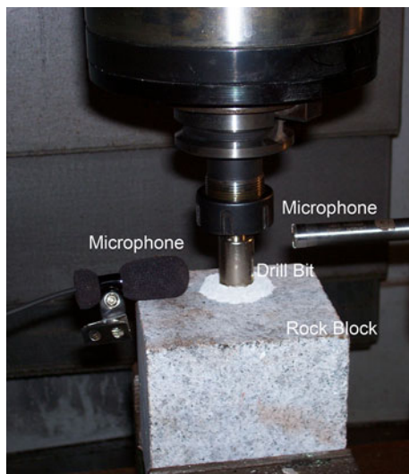
Fig. 2 Position of microphone from the drill setup
