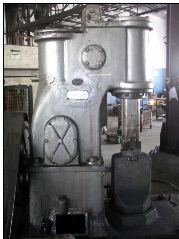
Fig. 2. Pneumatic power forging hammer.
