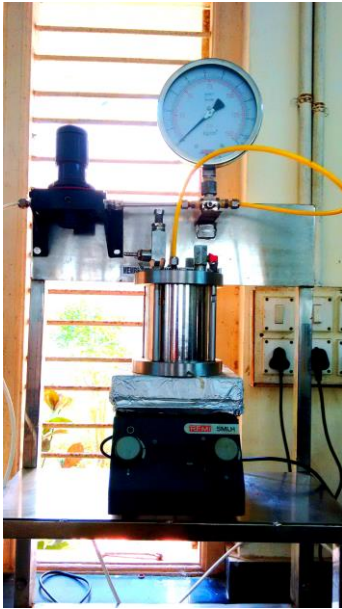
Batch system of membrane unit with Polytetrafluoroethylene (PTFE) membrane (10 cm dia, Axivia, India).
