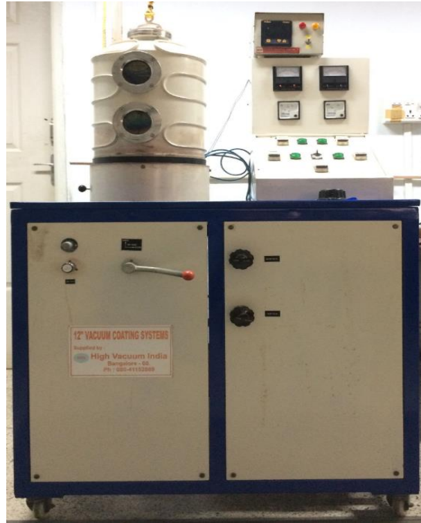
Figure 2.2 Photograph of thermal evaporation system used to prepare CdSe thin films.
