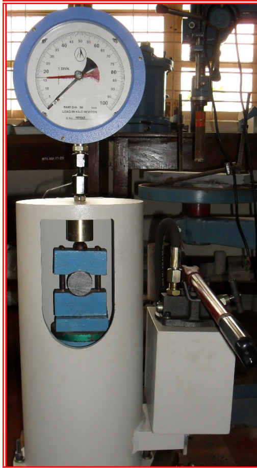
Fig 4.2 Brazilian Tensile Testing Machine
