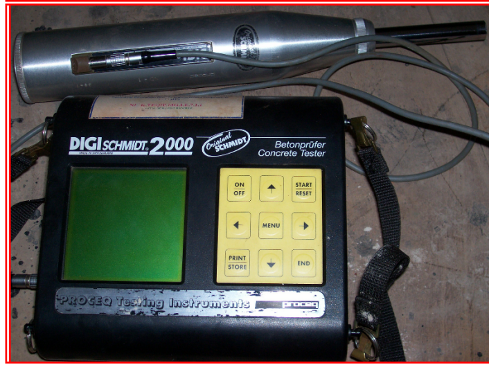
Fig.4.3 DIGI-SCHMIDT 2000, SRN measuring instrument
