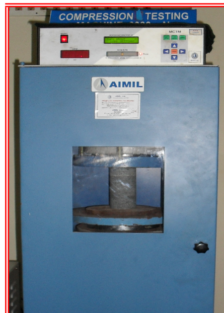
Fig.4.1 AIM-317E-Mu, Compression Testing Machine
