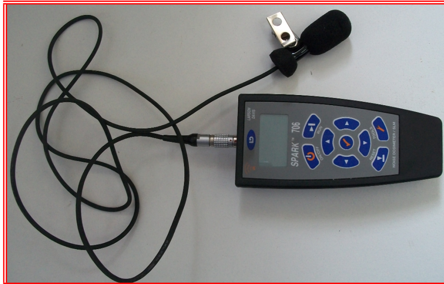
Fig. 4.4 Spark 706, Sound Measuring Instrument
