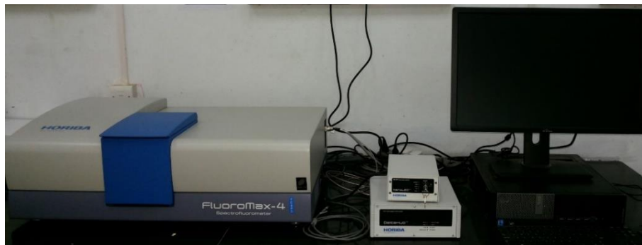
Figure 2.3 Fluoromax-4 TCSPC spectrophotometer for steady state and time resolved photoluminescence measurements
