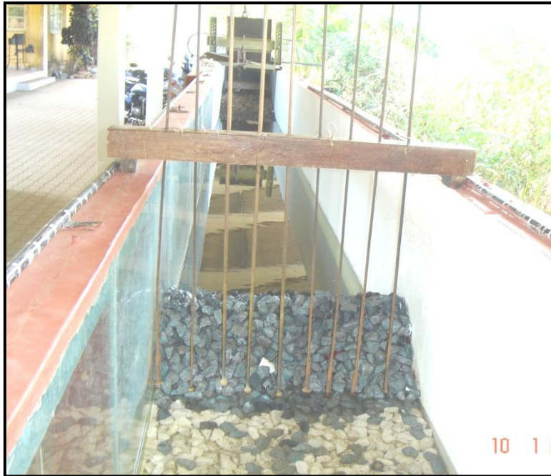
Plate 3.4 View of wave flume with profiler
