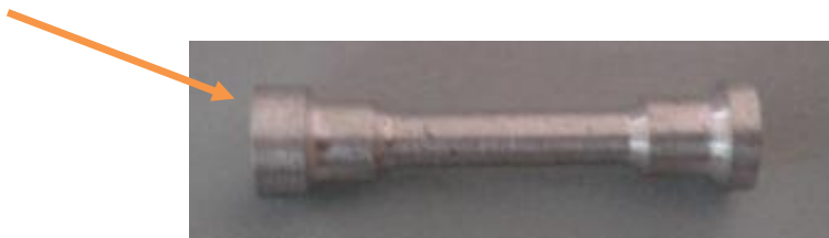
Figure 3.13 Specimen used for Testing the Tensile Strength using Electronic Tensometer
