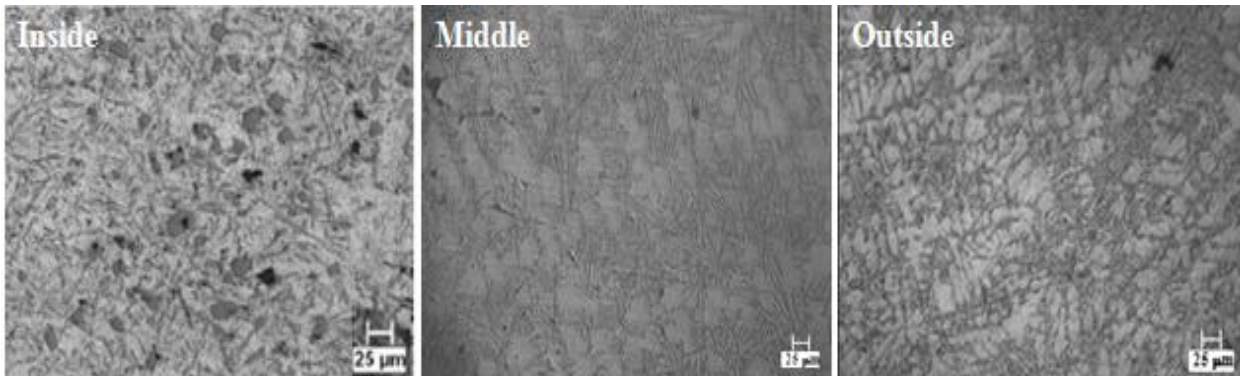
Figure 4.61 Microstructure of Al-12wt%Si Alloy cast at 600 rpm (14.9G)
