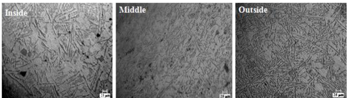
Figure 4.67 Microstructure of Al-17 wt % Si at 400 rpm (6.62G) of Rotational Speed of the mold
