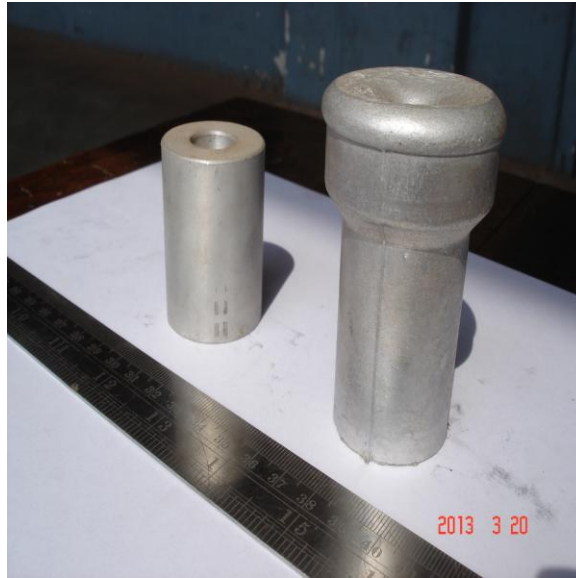
Fig.3.15 Photograph of a billet with 40 mm diameter and 50 mm height before and after machining
