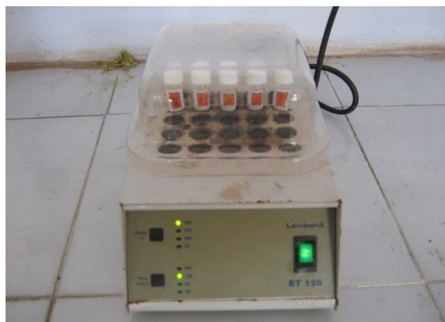
Fig. 3.5 COD digester used in the study
