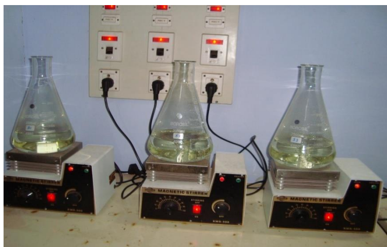
Fig. 3.1 Experimental Setup for Fenton's Oxidation of the Selected Pharmaceuticals
