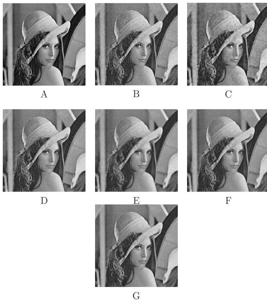
Figure 5.2: Image “Lena”:(A) Original image; (B) Blur and noisy image (out of focus blur: SNR 8dB); (C) After Applying Second-order shock proposed by Alvarez and Mazorra (1994); (D) After applying Fourth-order method proposed by You and Kaveh (2000); (E) After applying Fourth-order method proposed by Lysaker et al. (2003); (F)After applying method by Hajiaboli (2010); (G) After applying the FOEF Method.
