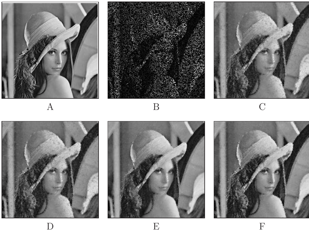
Figure 4.8: Image 'lena' (Original and reconstructed ones): (A) Original Image; (B) Image with data lost from random pixels (75%) and corrupted by a Gaussian noise with mean zero and variance: \sigma^2 = 0.01 (and blurred); (C) result of applying Perona-Malik method; (D) result of TV based method; (E) result of CDD method; (F) result of the proposed method.
