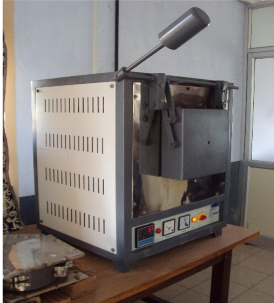
Figure 3.2: Muffle furnace with programmable temperature controller.
