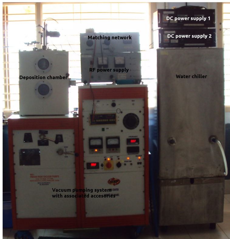
Figure 3.1: The DC and RF sputtering system
