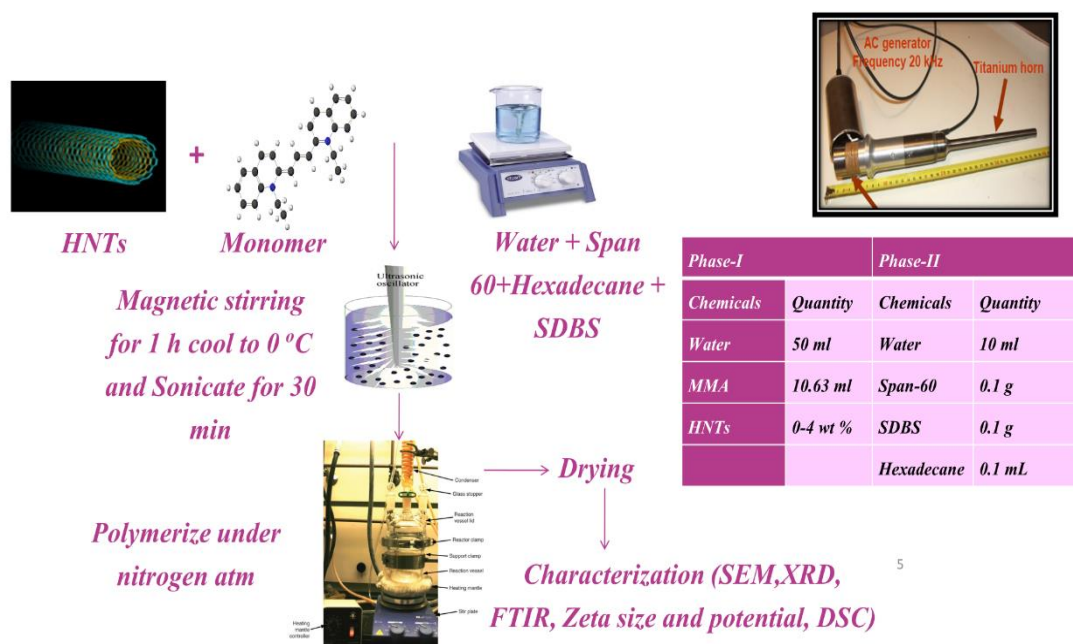
Figure 3.7 Synthesis of PNCs by miniemulsion polymerization
