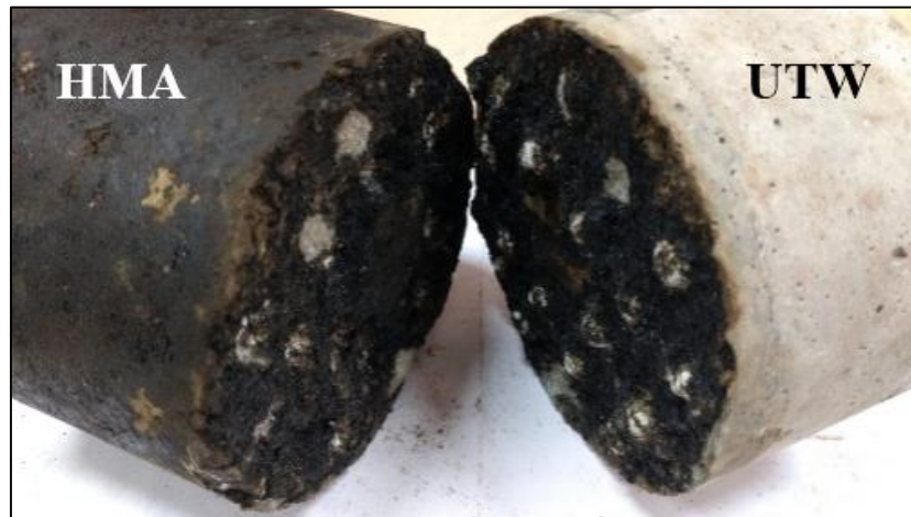
Fig. 3.16 Represents one of the HMA failed specimens with 100 % bonding interface
