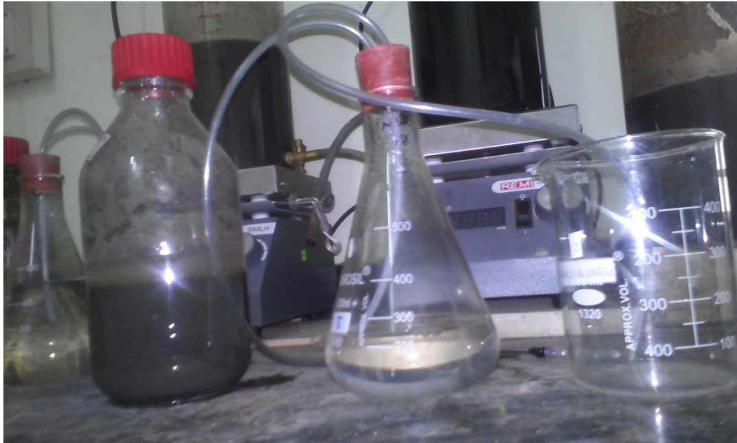
Figure 3.2 Batch digestion set-up
