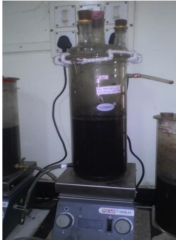
Figure 3.3 Semi-continuous mode digester set-up
