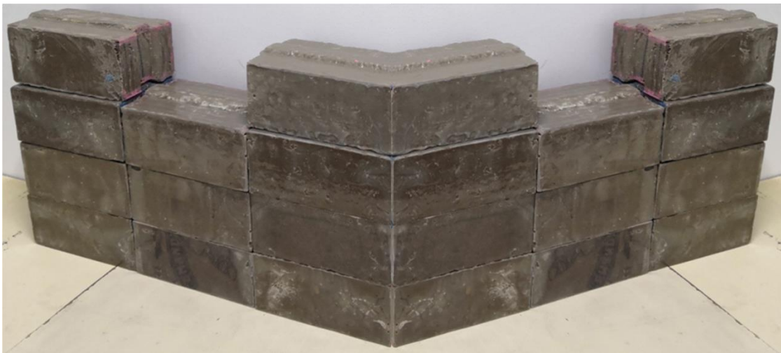
Figure 3. 47 Protective interlock blocks for bullet proofing
