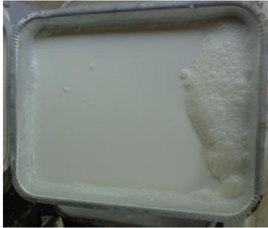
Figure 2.14 Natural rubber and formic acid mixture
