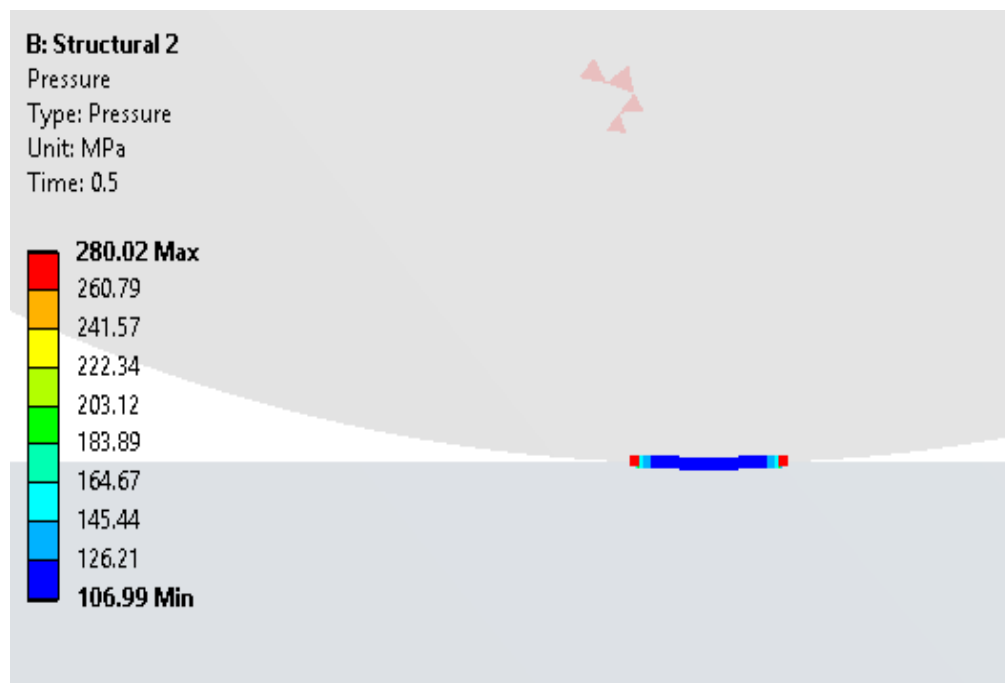
Figure 6.3 Contact Pressure Variation Between Elastic Cylinder and Flat Surface of 20F/5G/15B Composite.
