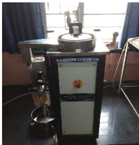
Figure 3.10 Pin on Disc Wear Test Setup (AIT, Pune)
