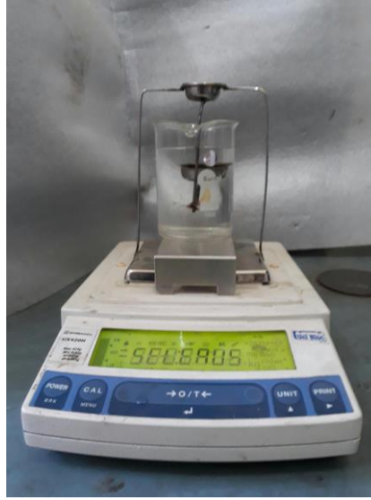
Figure 7.10 Densitometer for measuring density of acrylic plate
