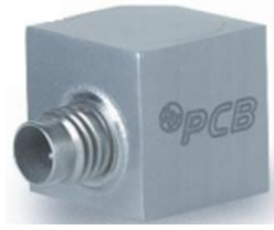
Figure 6.7. Accelerometer for measuring the vibration
