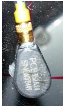
Figure 7.6 Accelerometer for measuring the vibration
