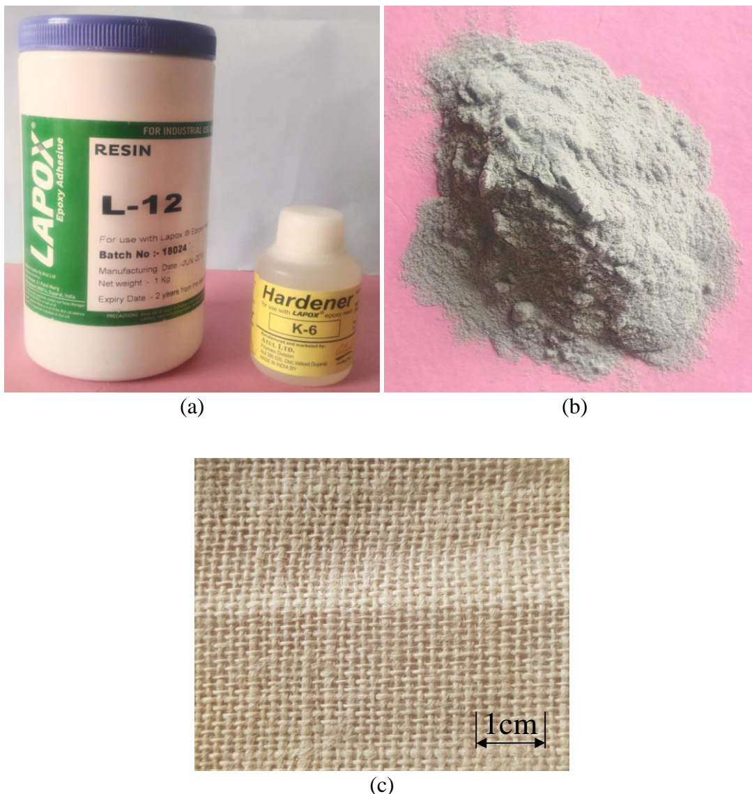
Figure 2.1 (a) Epoxy resin and hardener (b) Cenospheres and (c) Sisal woven fabric used in this study.
