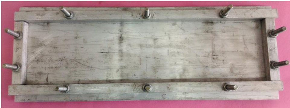
Figure 2.2 Aluminium mold used to prepare syntactic foams.
