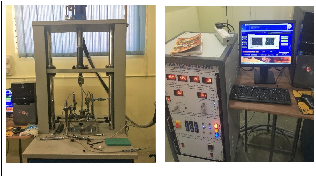
Figure 4.18 Fatigue test set up
