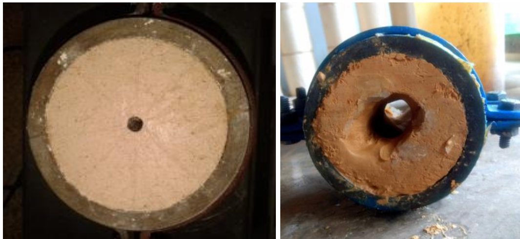
Figure 5.1. (a) Sample before test with 6mm hole (b) Sample(C10) which showed very less surface erosion after HET when coated with wax on its surface
