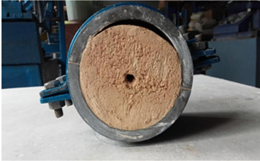
Figure 5.27. Sample which collapsed when compacted to 90% wet of optimum
