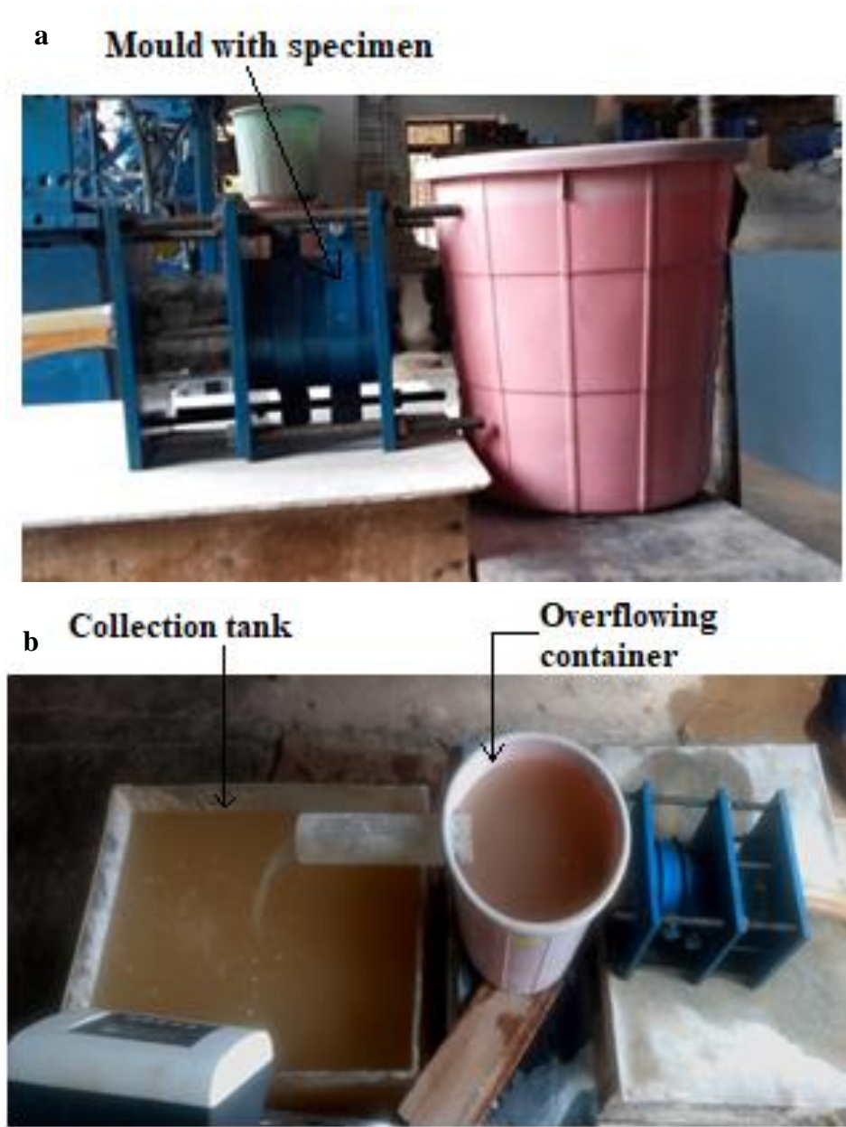
Figure 3.3. Hole Erosion Test apparatus (without constant head tank) a) Front view b) Top view
