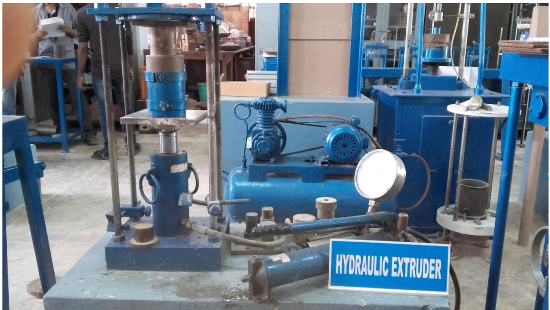
Figure 3.4. Preparation of sample using a hydraulic extruder
