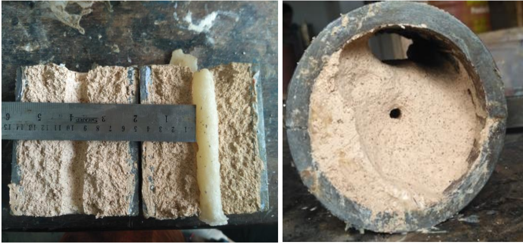
Figure 5.2. (a) Cross section of a sample after HET (b) Formation of second hole due to slaking
