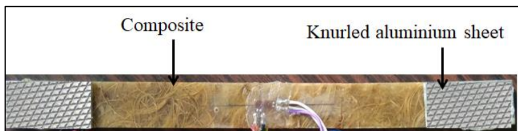
Figure 4.1 Test specimen pasted with knurled aluminium sheet.
