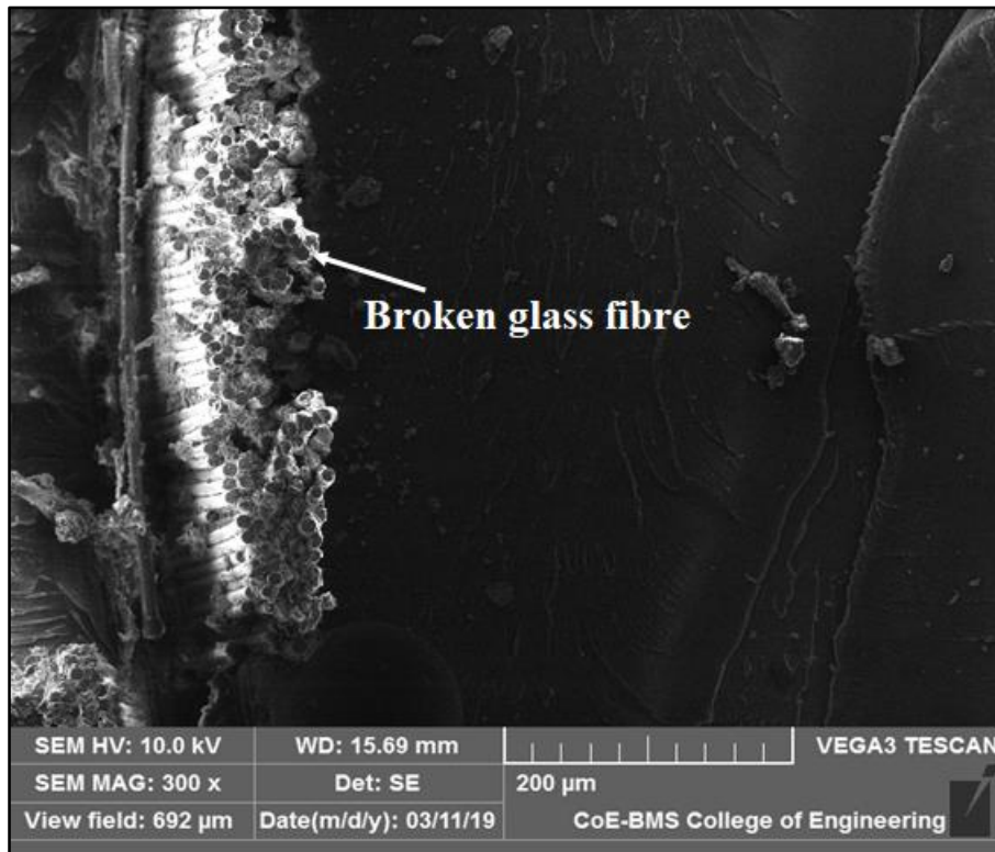
Figure 4.36 SEM micrographs of composites made with CF+GF after flexure test.
