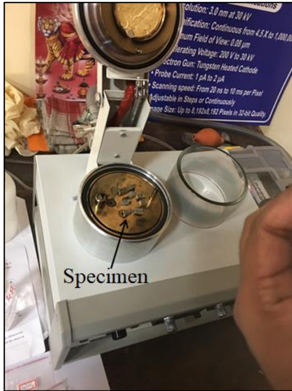
Figure 4.29 Specimens arranged for sputter coating.
