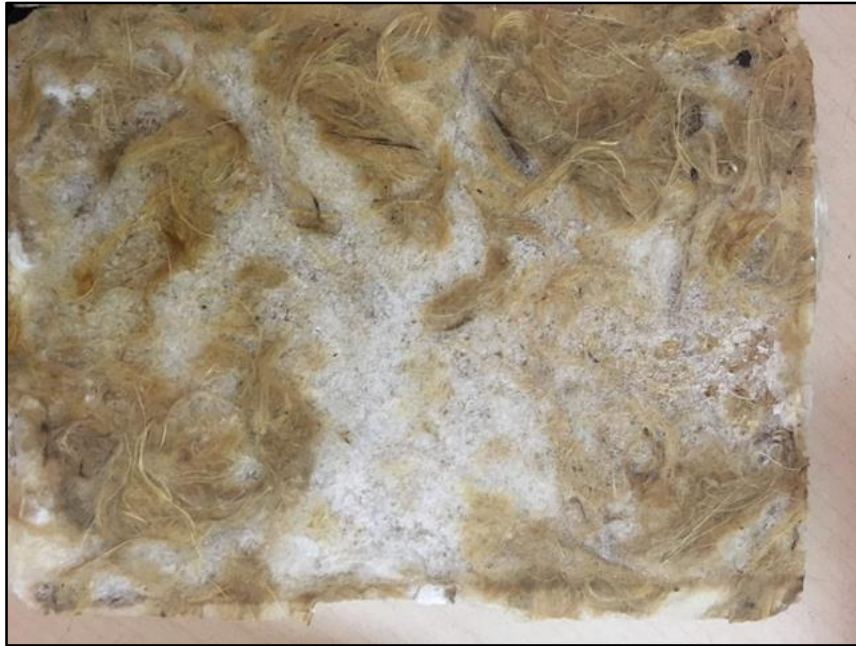
Figure 2.17 Failure of AHF composite panel due to hot press moulding.
