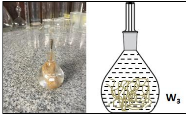
Figure 2.4 Pycnometer with arecanut husk fibre and water.
