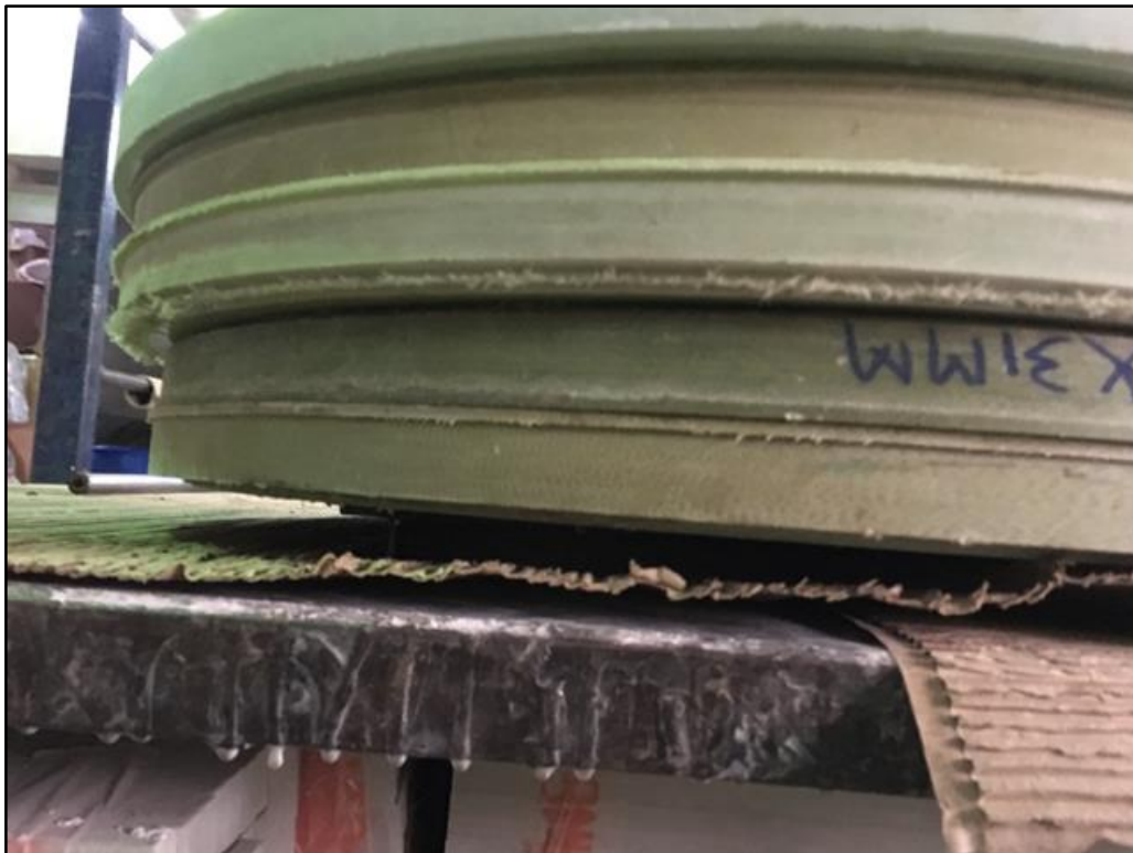
Figure 2.22 Application of uniformly distributed load on mould.
