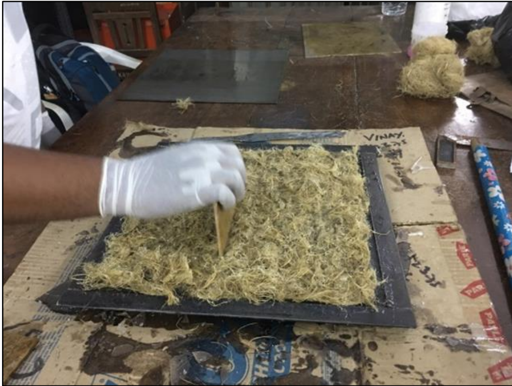
Figure 2.21 Random arrangement of fibre in mould.
