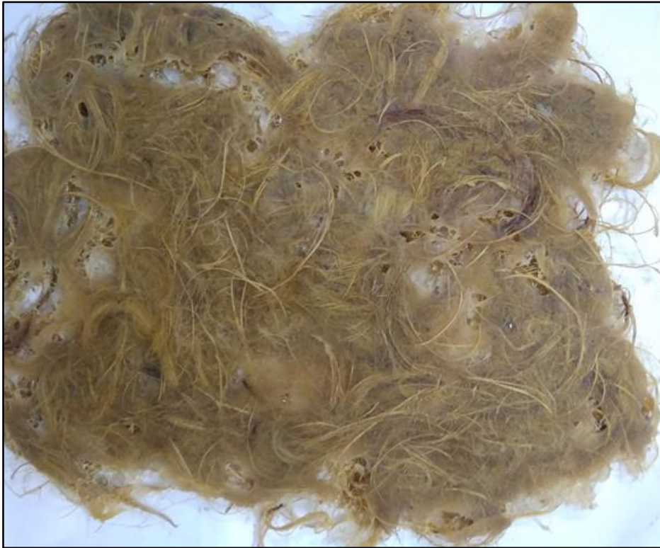
Figure 2.19 Failed cast panel due to uneven distribution of epoxy resin.
