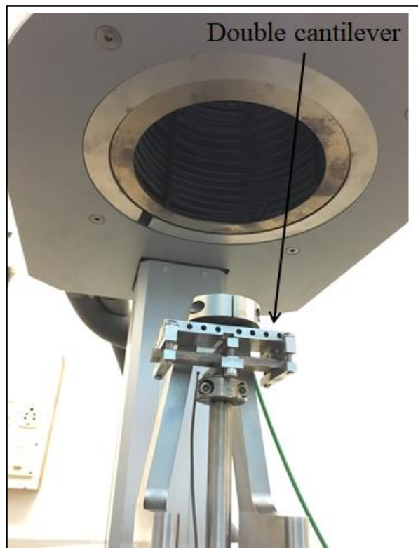
Figure 3.7 Double cantilever beam arrangement in DMA.
