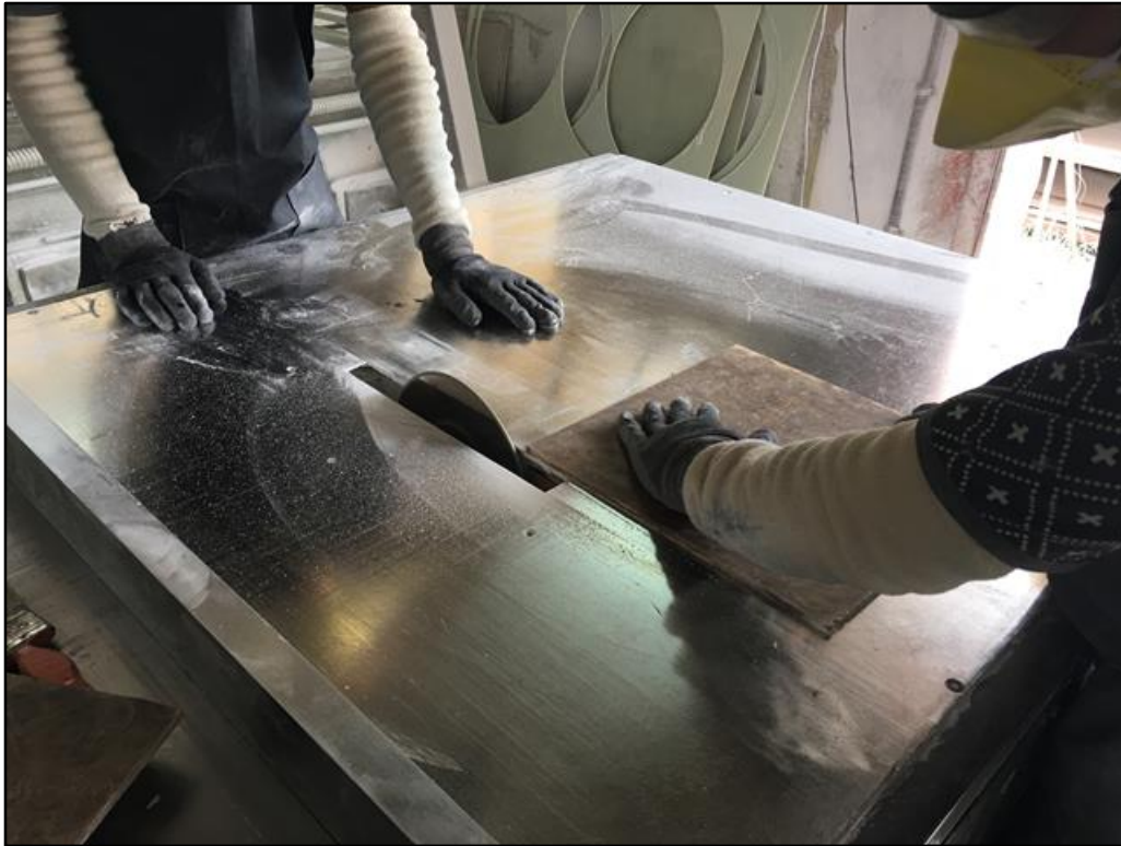
Figure 3.5 Specimen cutting process using diamond cutter.
