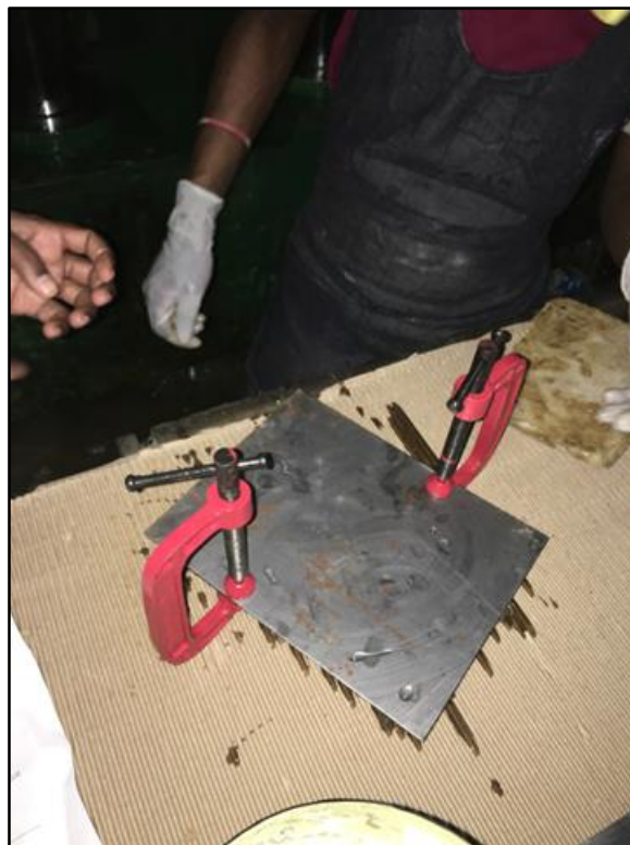
Figure 2.18 Holding cover plate of cast mould with C-clamps.
