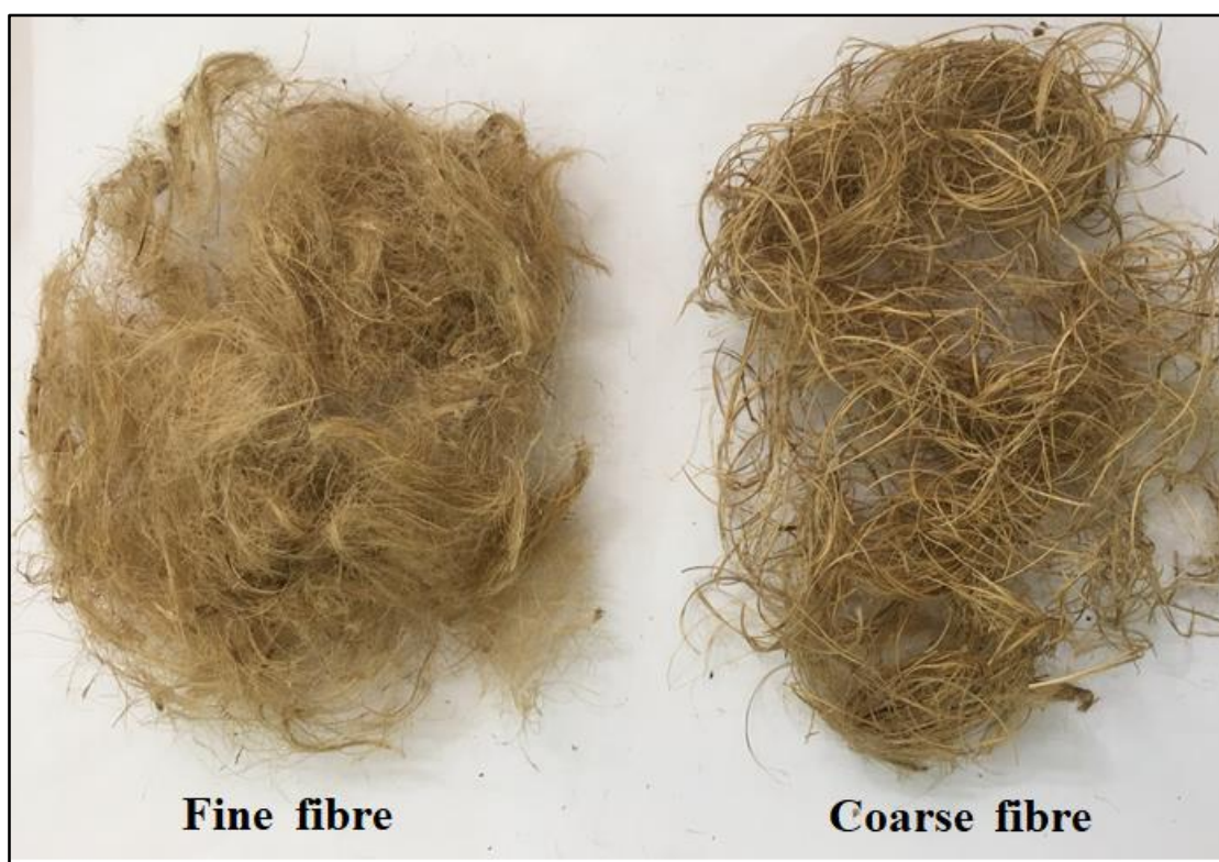
Figure 2.11 Extracted fibre from arecanut husk.
