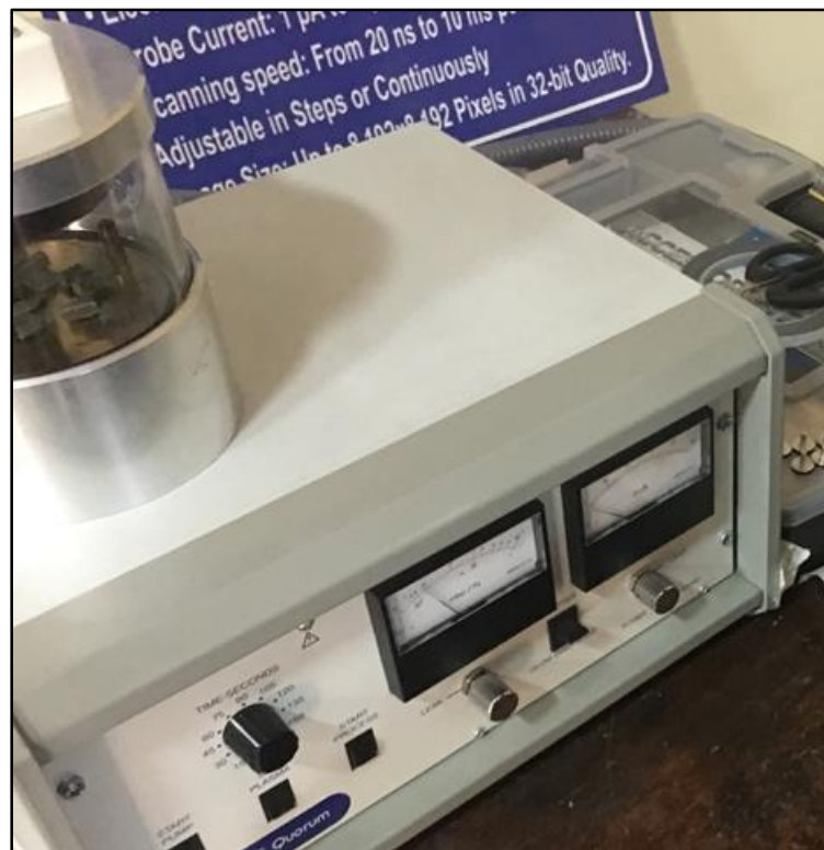
Figure 4.30 Sputter coater during coating process.
