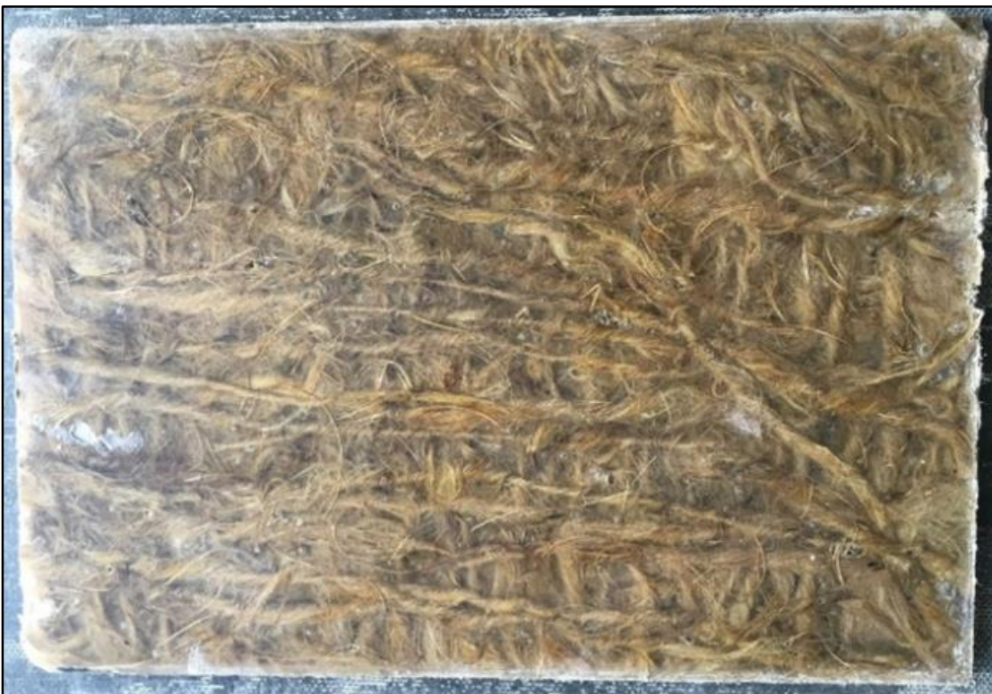
Figure 3.4 Cast arecanut husk fibre epoxy composite panel.
