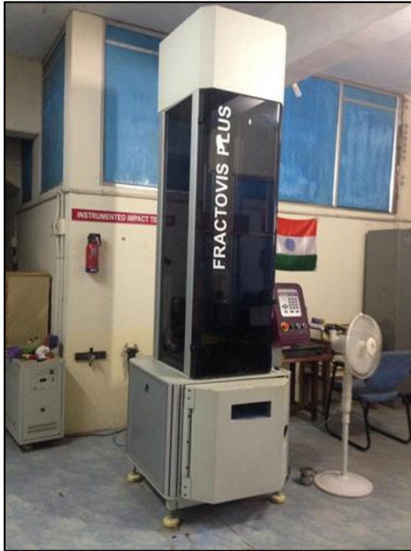
Figure 4.17 Fractovis plus drop weight impact testing machine.
