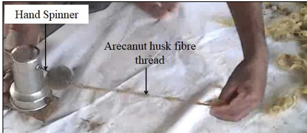
Figure 3.1 Preparation of arecanut husk threads using hand spin yarning process.
