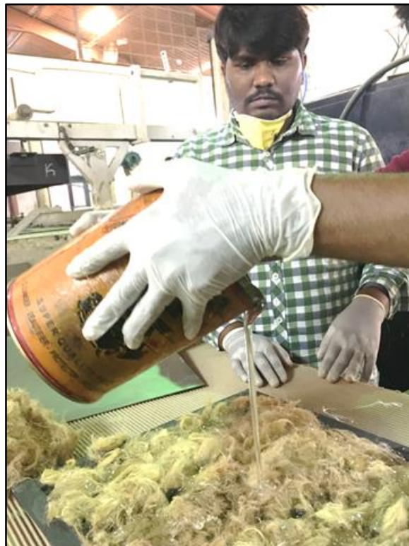
Figure 2.16 Addition of epoxy resin to the fibre.
