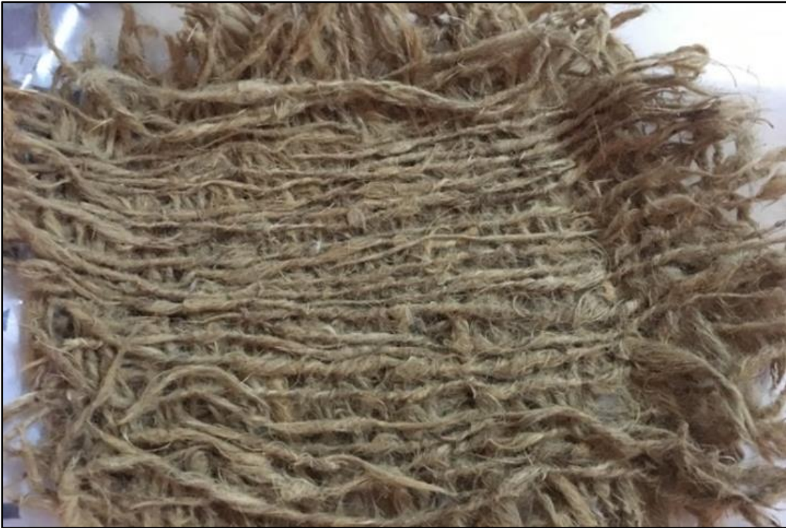
Figure 3.3 Arecanut husk fibre threads orientation in the form of mat for specimen preparation.
