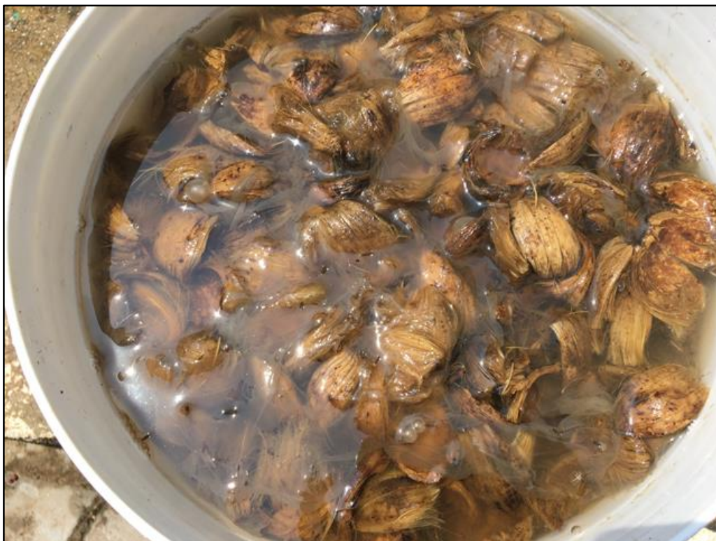
Figure 2.9 Soaking arecanut husk in alkaline solution.
