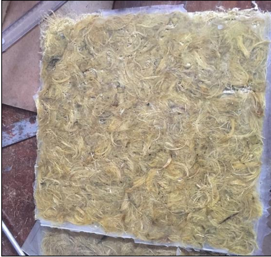
Figure 2.23 AHF composite panel after unmould.
