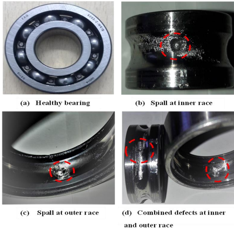
Figure 3.11 Ball bearing conditions used in the GB (a) Healthy, (b) Spall at inner race, (c) Spall at outer race, (d) Combined defects at inner and outer race
