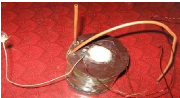
Figure 5. Solenoid for actuation of Terfenol D.
