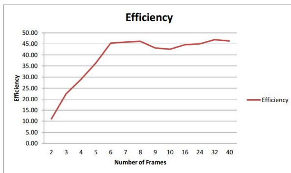
Figure 8. Graph showing Efficiency of parallel registration module.
