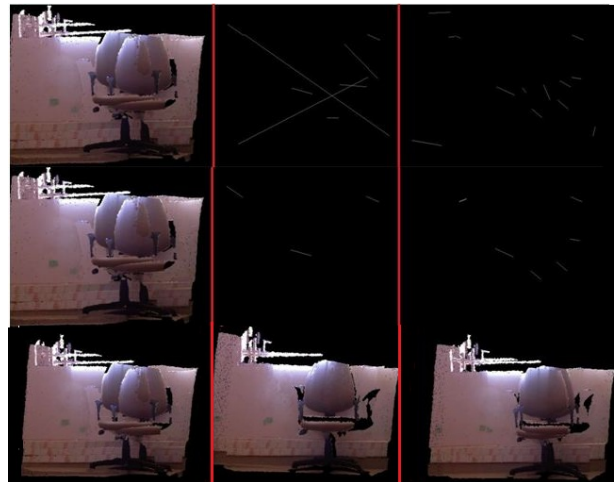
Figure 4. Comparison of methods of finding correspondence between two clouds using FPFH descriptor and using SIFT keypoints.
