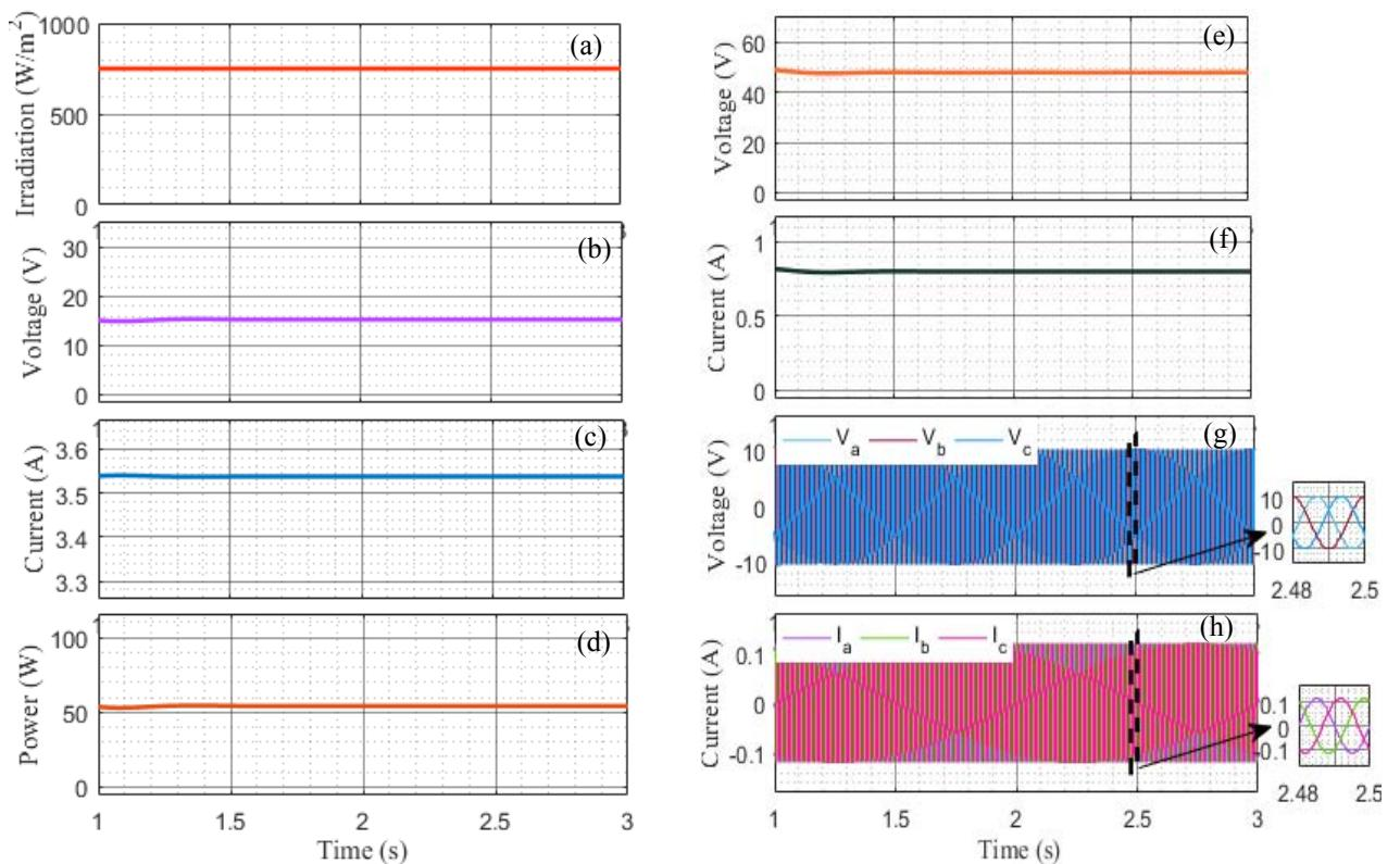
Fig. 7. Performance of hybrid power converter in non-MPP mode at constant irradiation ( $750 \text{ W/m}^2$ ). (a) Irradiation. (b) PV panel voltage. (c) PV panel current. (d) PV power, (e) DC output voltage (f) DC output current. (g) 3 phase AC output voltage, (h) 3 phase AC output current.
