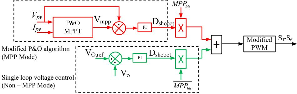
Fig. 3. Control block diagram of the proposed hybrid power converter
