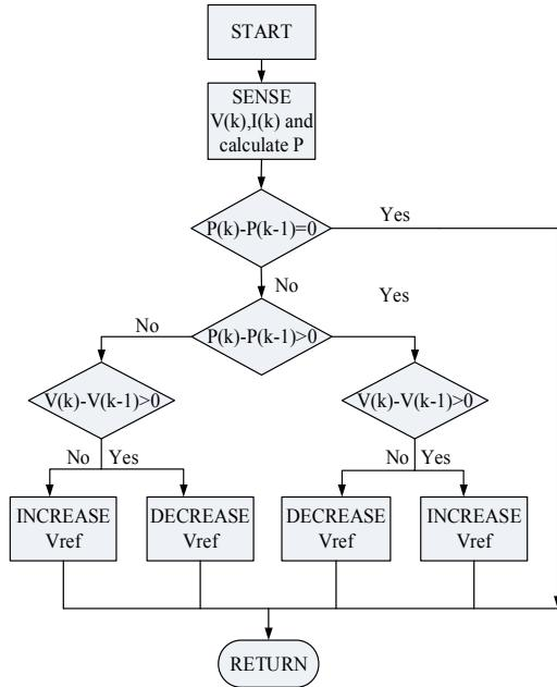
Fig. 4b. MPPT algorithm flowchart
