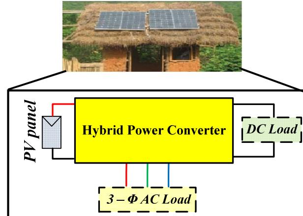
Fig. 1. Rural home with PV fed hybrid converter
