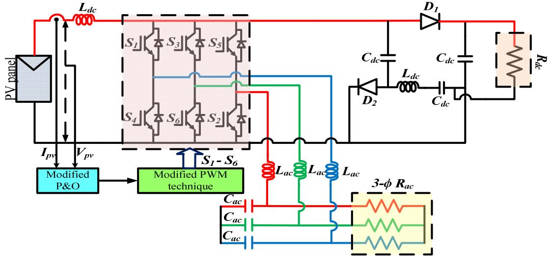
Fig. 2 Control block diagram of the proposed hybrid power converter
