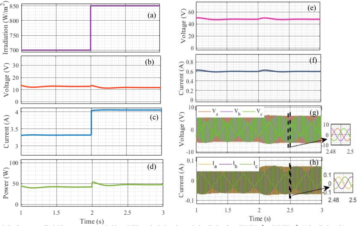
Fig. 8. Performance of hybrid power converter in Non - MPP mode during change in irradiation from  $700 \text{ W/m}^2$  to  $850 \text{ W/m}^2$ . (a) Irradiation. (b) PV panel voltage. (c) PV panel current. (d) PV power, (e) DC output voltage (f) DC output current. (g) 3 phase AC output voltage, (h) 3 phase AC output current.
